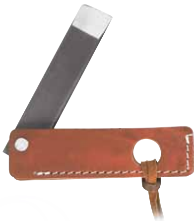
Part # 44150 Mult-Purpose Sharpening Steel Tungsten carbide bonded to fine, medium and rough surfaces can sharpen any blade. The chisel point is useful for other jobs that would harm a knife such as prying, chiseling, scrapping or splitting.
