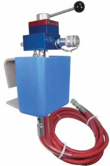
Part # TEHIS-810 Hydraulic Intensifier This intensifier increases the pressure of the hydraulic system of a vehicle so that high-pressure tools can be operated without an additional power unit. It operates on either open or closed center systems and has an optimum operating pressure of 1,800 psi at 6 gpm. Flow range is 4 - 7 gpm. Includes a 10' non-conductive, low-pressure twin-line hose and 8' of high-pressure hose.
