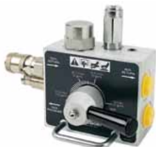
Part # HFC30 Hydraulic Flow Control Valve Operates off of a vehicle's hydraulic circuit. It can accept a flow of up to 30 gpm and reduce it to a maximum of 10 gpm allowing the correct flow to the hydraulic tool.
