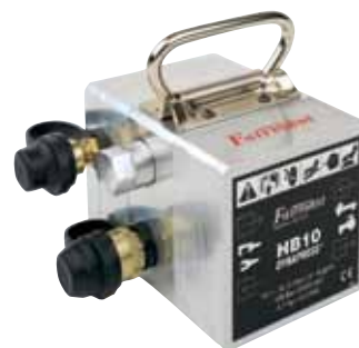
Part # HB10 Hydraulic Intensifier Works on both open and closed center systems and produces 10,000 psi. Input pressure is from 1,000 to 2,000 psi and has a flow rate between 4 - 8 gpm. Couplers & hose sold separately.
